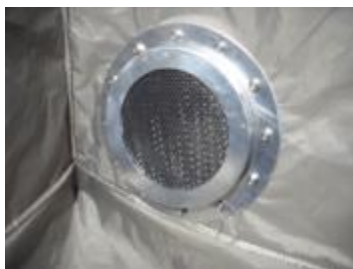
Inside of Air-Filing hole/honeycomb
