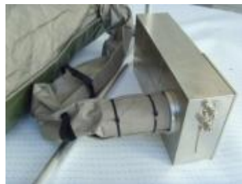
Power-tube / EMI filter box Connection
